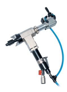
The FM-1625 auto lock machine suitable for high volume repetitive works on heat exchangers and condensers etc. The automatic locking feature dramatically reduces production time. It produces fast accurate weld preps on any schedule and material of pipe effortlessly within its range.
